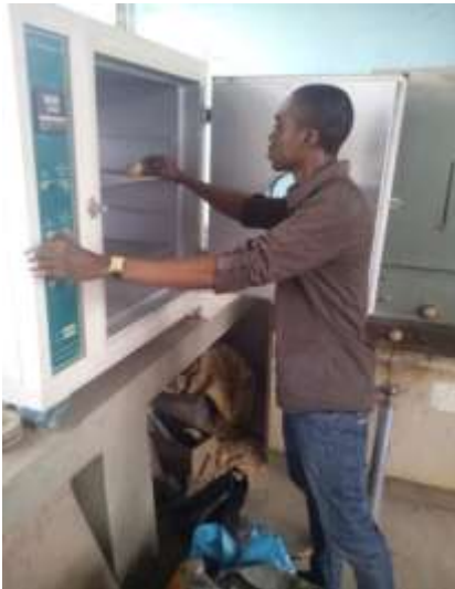
Fig. 3: Drying of moisture content cans using electric oven
